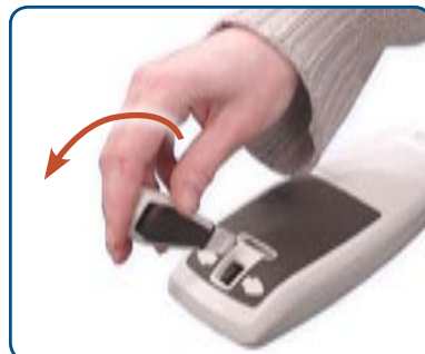
Fig. 2/20: Remove the joystick, if required
