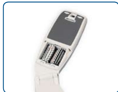
Fig. 4/2: Control unit batteries.
