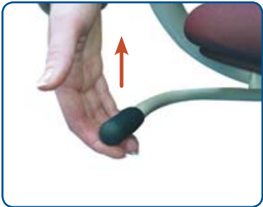
Fig. 2/14: Manual seat swivel handle.
