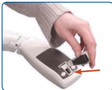
Fig. 2/3: Inserting the joystick
