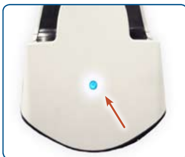
Fig. 2/5: Status lamp on the motor cover
