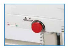
Or the secondary set of controls with emergency stop mounted on the control box. Control box also has a built-in cycle counter.
