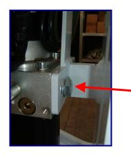
7) Remove the oleodinamic panel from the right side -back view. Warning: Do not turn the oleodinamic panel upside down in order to avoid oil leaks.
