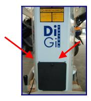
3) Unscrew the 2 screws at the lateral sides of the main chassis.
