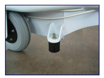
In case of more relevant slopes closet o the pool deck, you have to cut the rubber stoppers in order to make them shorter. In this way the lifter gets smooth to the pool deck. Use a cutter to cut the rubber stoppers.
