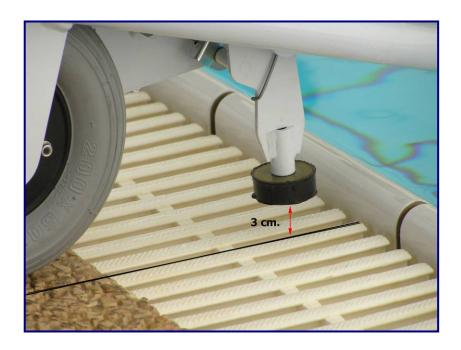
If the distance is more than cms. 3, unscrew the rubber part of the endings and add one or more nuts in order to reach the correct distance of cms. 3 from the ground.
