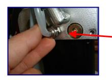
4) Unscrew the screw and remove the electric valve connection – red colour
