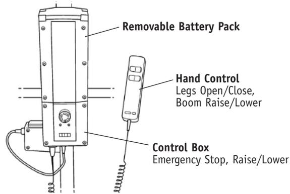
When the power pack needs charging it is removed from the lift and fitted to an off board charging unit.
